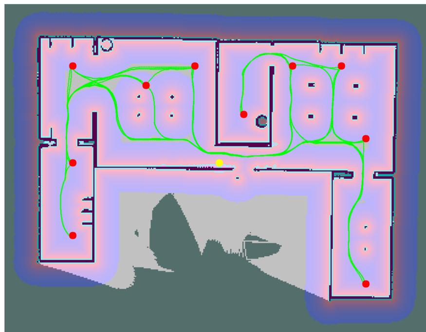
**Figure 5.** Map of the environment, cost map, start points and stop points marked with red, initial planned paths marked with green, and the origin of the coordinate system marked with yellow.
