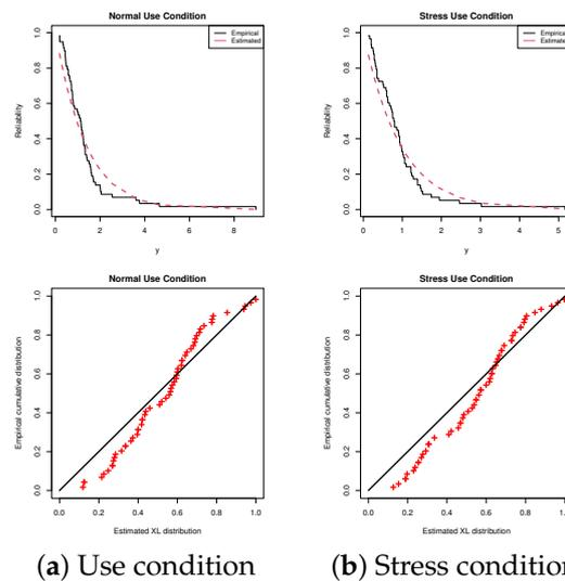
**Figure 10.** Fitted reliability (left) and PP (right) plots from LED data.
