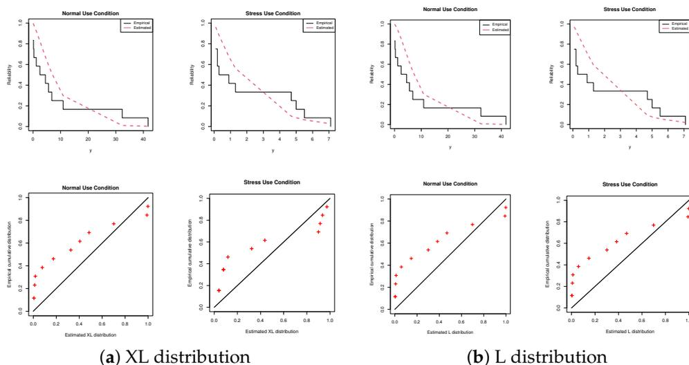
**Figure 6.** Fitted reliability (top) and PP (bottom) plots from insulating fluid data.
