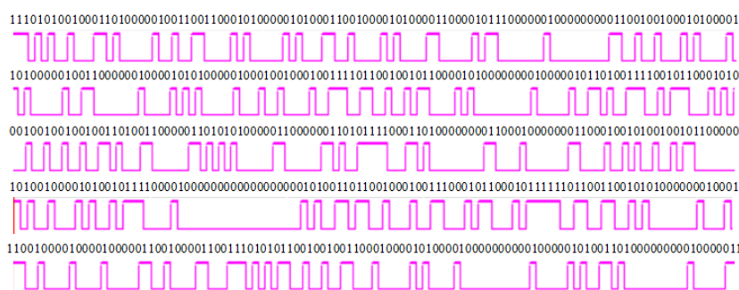
Figure 4. Restart experiment with 100 initial values captured through a logic analyser interfaced with an FPGA.
