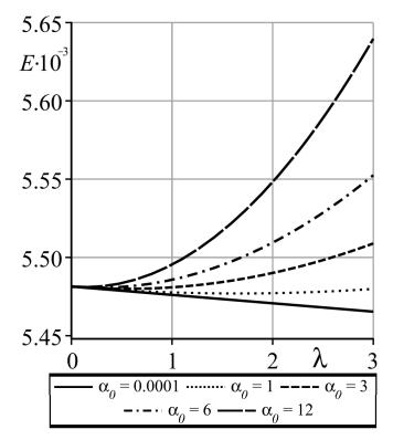
**Figure 11.** Plots of the contact energy loss *E* versus  $\lambda$  for different values of  $\alpha_0$ .
