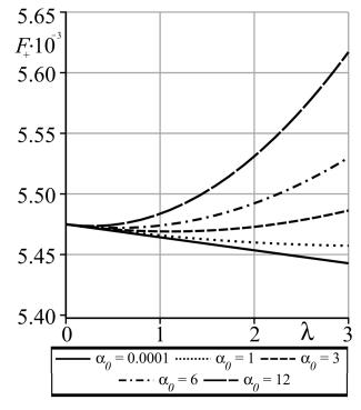
**Figure 9.** Plots of the friction force  $F_+$  versus  $\lambda$  for different values of  $\alpha_0$ .
