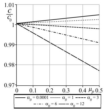
**Figure 4.** Plots of the dependence of the relative lubricated contact exit coordinate  $c/c_0$  versus  $\mu_p$  for different values of  $\alpha_0$ .
