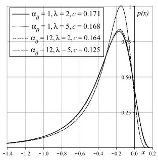
**Figure 2.** Plots of contact pressure distributions p(x) for the basic set of input parameters and different values of  $\alpha_0$  and  $\lambda$ .
