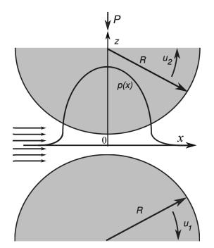
Figure 1. The general view of a lubricated contact.
