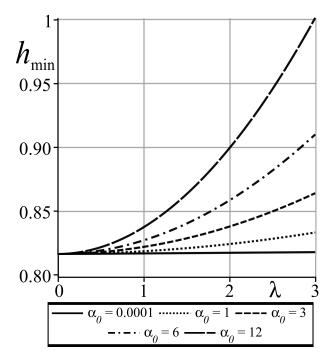
**Figure 7.** Plots of the dependence of the minimum lubrication film thickness  $h_{min}$  versus  $\lambda$  for different values of  $\alpha_0$ .
