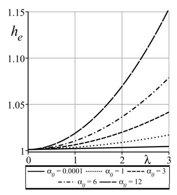
**Figure 5.** Plots of the dependence of the exit lubrication film thickness  $h_e$  versus  $\lambda$  for different values of  $\alpha_0$ .
