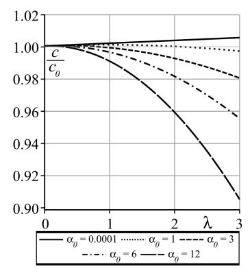
**Figure 3.** Plots of the dependence of the relative lubricated contact exit coordinate  $c/c_0$  versus  $\lambda$  for different values of  $\alpha_0$ .
