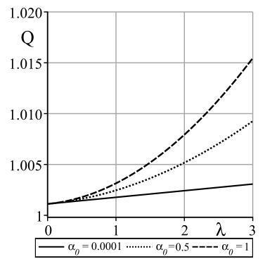
**Figure 12.** Plots of the lubricant volume flux *Q* versus  $\lambda$  for different values of  $\alpha_0$ .
