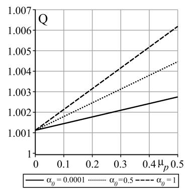
**Figure 13.** Plots of the lubricant volume flux *Q* versus  $\mu_p$  for different values of  $\alpha_0$ .
