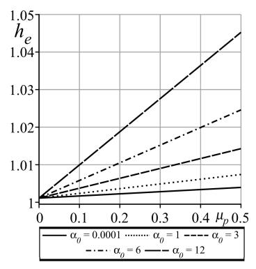
**Figure 6.** Plots of the dependence of the exit lubrication film thickness  $h_e$  versus  $\mu_p$  for different values of  $\alpha_0$ .
