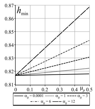
**Figure 8.** Plots of the dependence of the minimum lubrication film thickness  $h_{min}$  versus  $\mu_p$  for different values of  $\alpha_0$ .
