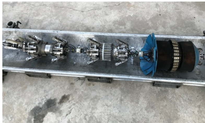
Figure 7. Magnetic flux leakage detector.
