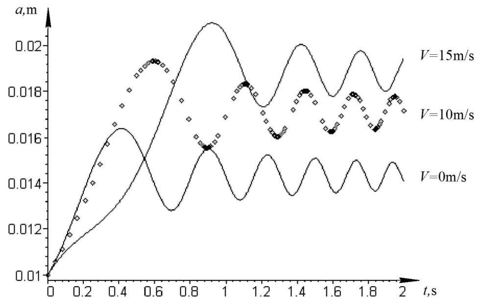
**Figure 6.** Resonance amplitude curves in the transition process at different longitudinal velocities of the beam ( $V = 0$  m/s,  $V = 10$  m/s,  $V = 15$  m/s).
