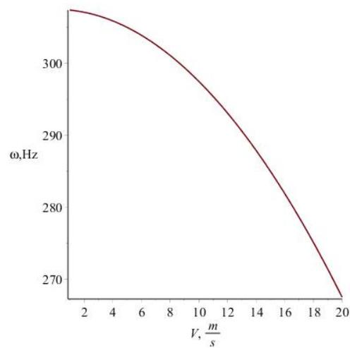
**Figure 3.** The effect of longitudinal velocity of the beam on vibration frequency (with fixed initial vibration amplitude of 0.01 m).
