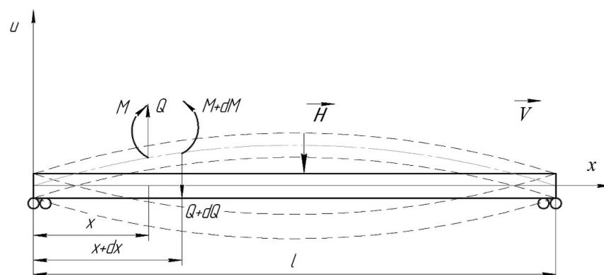
Figure 1. Schematic model of a beam moving along its axis.
