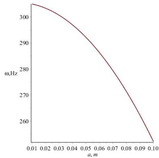
**Figure 4.** The effect of amplitude on vibration frequency of the beam (with longitudinal velocity fixed at 5 m/s).
