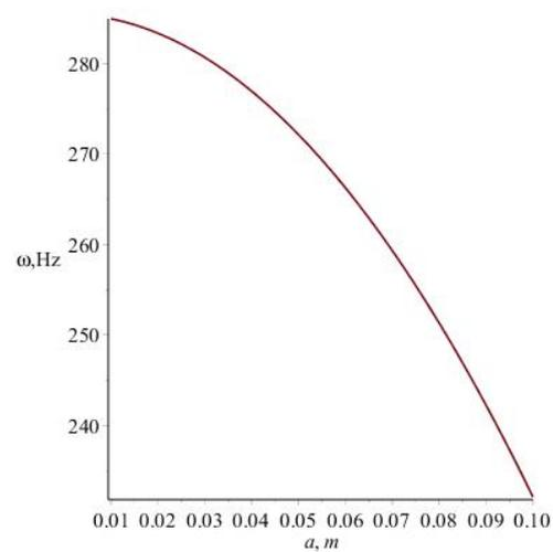
**Figure 5.** The effect of amplitude on vibration frequency of the beam (with longitudinal velocity fixed at 15 m/s).
