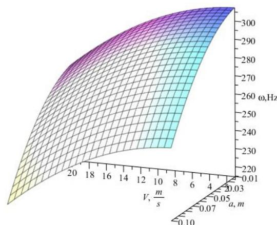
Figure 2. The effect of amplitude and longitudinal velocity of the beam on vibration frequency.
