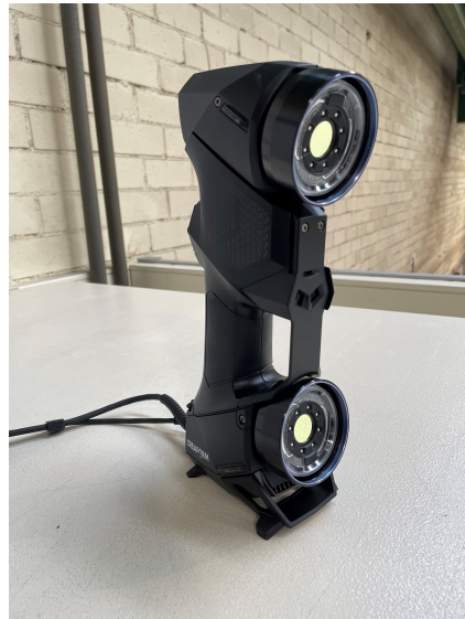
Figure 3. Three-dimensional (3D) laser scanner used for the measurement of displacements of the samples during the cyclical freeze–thaw temperature load.
