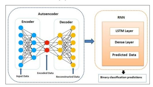
Figure 4. The RNN autoencoder architecture for SQL injection attack detection.
