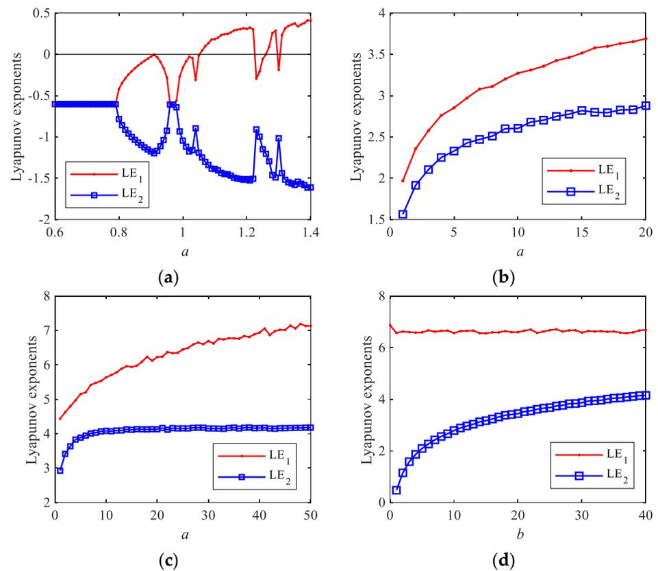
**Figure 3.** Lyapunov exponent graph of three 2D chaotic maps: (a) Lyapunov exponent of Hénon map; (b) Lyapunov exponent of 2D-SLG map; (c) Lyapunov exponent of the proposed map versus parameter  $a$ ; (d) Lyapunov exponent of the proposed map versus parameter  $b$ .
