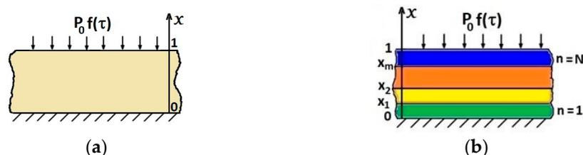
**Figure 1.** Loading of the layer’s cross section. (a) FG layer; (b) piecewise-homogeneous layer.
