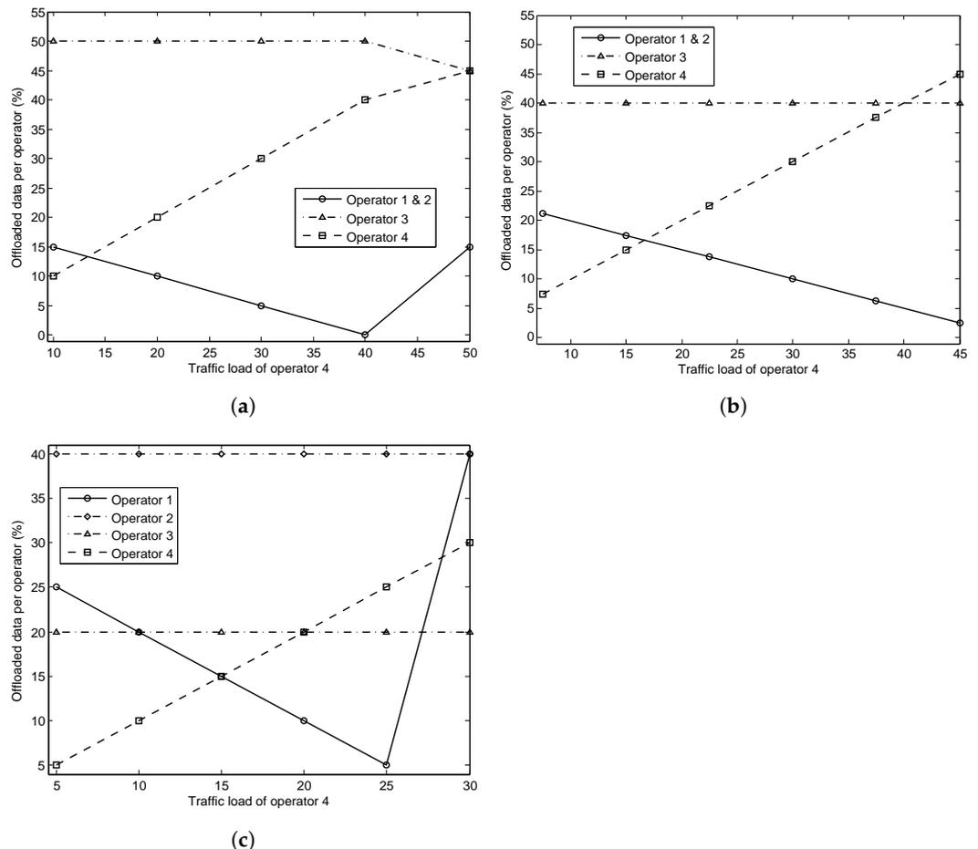
**Figure 6.** Impact of network traffic on the offloaded data of each operator. (a) Scenario 1—High traffic; (b) Scenario 2—Medium traffic; (c) Scenario 3—Low traffic.
