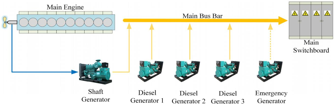
Figure 2. A general illustration of the ship’s microgrid.
