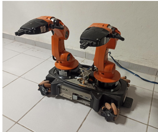
Figure 1. Mobile dual-arm system KUKA® Youbot®. It is composed of two 5-DOF manipulators and a 3-DOF mobile platform.
