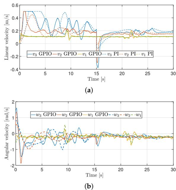
**Figure 15.** Control inputs for the robots for the second experiment. (a) Longitudinal velocities. (b) Angular velocities.
