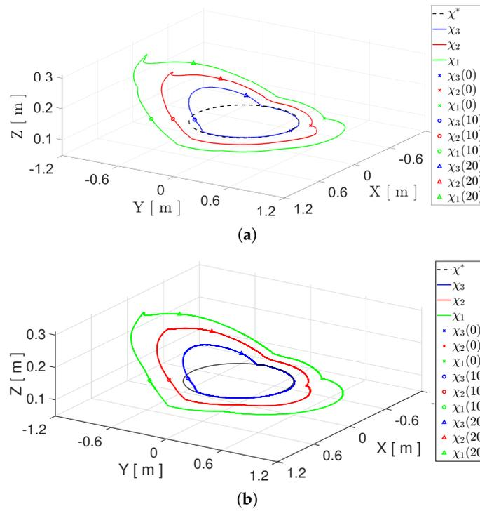
**Figure 10.** Trajectory in the three dimensional space of the mobile robots for the second experiment. (a) Trajectory in the three dimensional space with the GPIO approach. (b) Trajectory in the three dimensional space with the PI approach.
