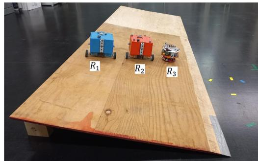
**Figure 9.** Uneven surface as a disturbance experimental test.
