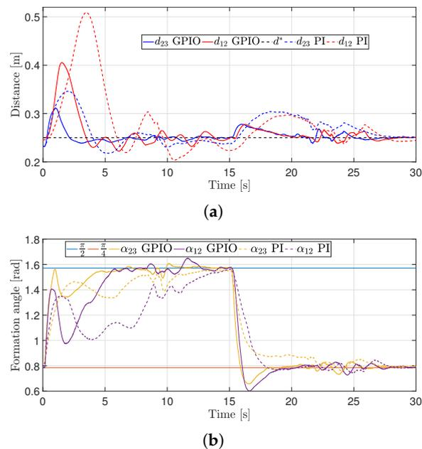
**Figure 13.** Distances and formation angles between the robots for the second experiment. (a) Distances between the robots. (b) Formation angles between the robots.
