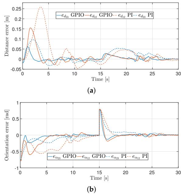
**Figure 14.** Distances and orientation angles errors for the second experiment. (a) Distance error. (b) Orientation error.
