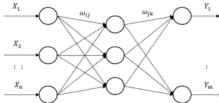
Figure 2. BP neural network topology diagram.
