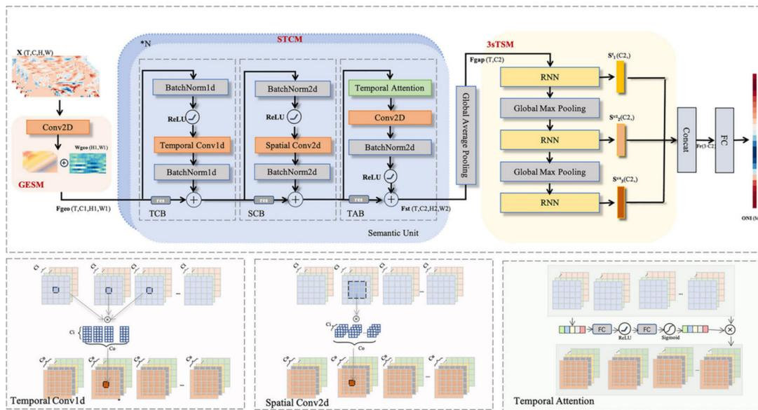
Figure 5. The pipeline of the proposed STSNet [54].
