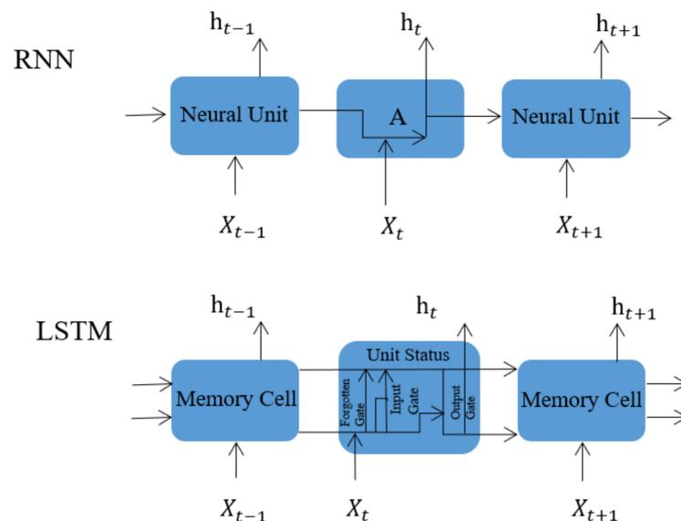
Figure 6. Comparison of the RNN and LSTM structure.
