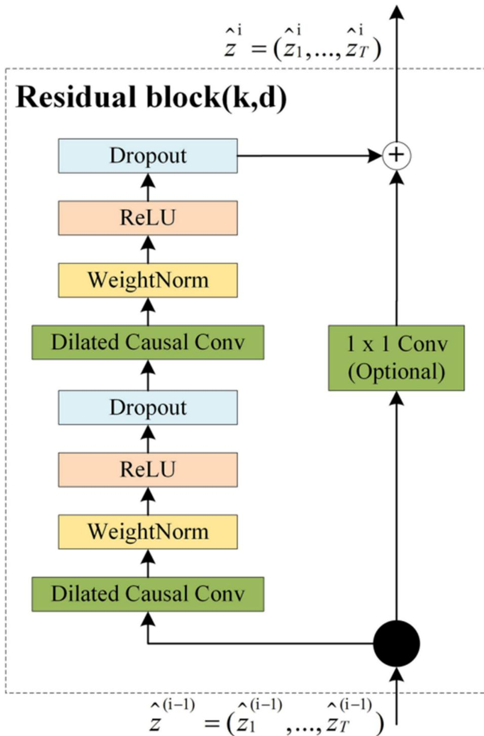
Figure 4. The TCN residual module [52].
