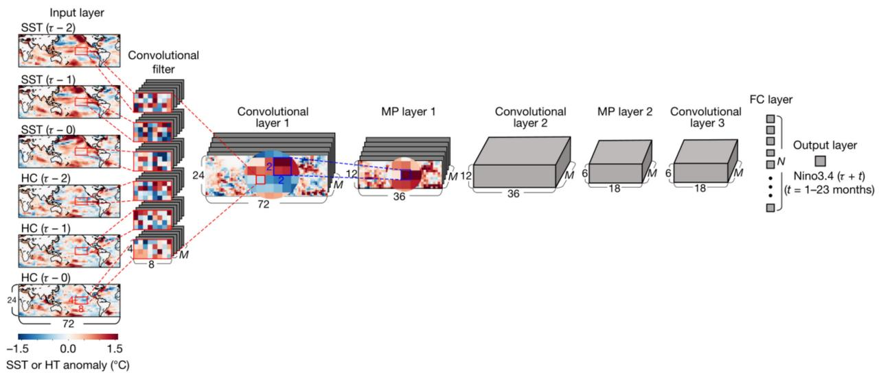
**Figure 3.** Structure of the CNN model for ENSO prediction [51].
