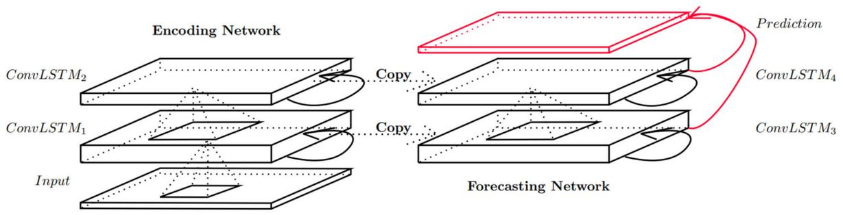
Figure 7. Encoding-forecasting ConvLSTM network [63].
