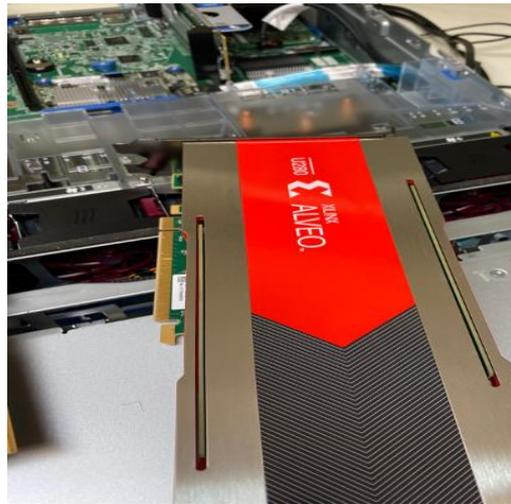
**Figure 7.** Xilinx Alveo U280 accelerator card.
