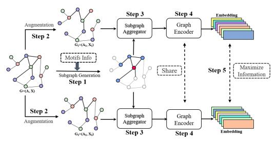
**Figure 2.** The over all architecture of the proposed PASCAL for unsupervised node classification, which uses feature masking as augmentation strategy. The model mainly consists 5 components: (1) subgraph generator; (2) augmentation; (3) subgraph aggregator; (4) graph encoder; and (5) comparator.
