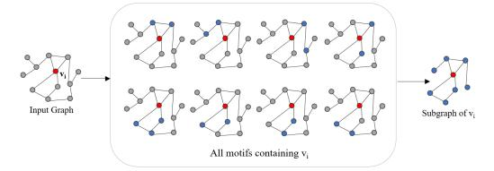
**Figure 3.** The process of generating subgraph for node  $v_i$  on the basis of its motif information. The red node represents the target node  $v_i$  and the blue nodes represent the nodes that appear in the same motif as  $v_i$ . For all networks in the middle box, the blue and red nodes represent all motifs containing the target node.
