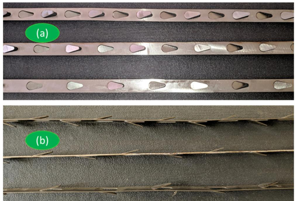
**Figure 3.** (a) Top View of the PWT with different pitches (b) Side view of the PWT with different inclinations [29].
