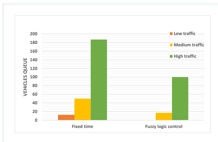
Figure 8. The comparison of average intersection considering the different conditions without a controller and with a controller.
