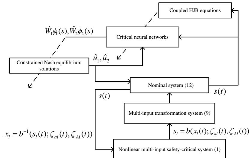
Figure 1. The structure diagram of the proposed multi-input safety-critical system.
