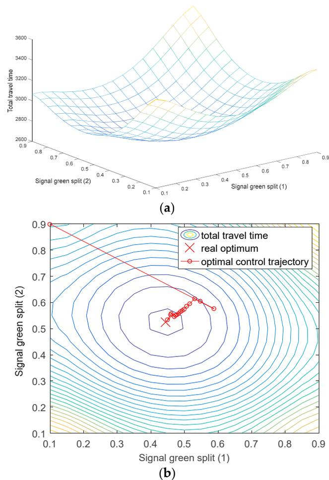
**Figure 3.** The optimal control trajectory in total travel time contours. (a) The total travel time surface. (b) The optimal control trajectory.
