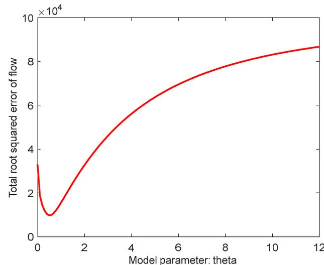
Figure 7. Summation of root squared error of flow under all feasible control settings.
