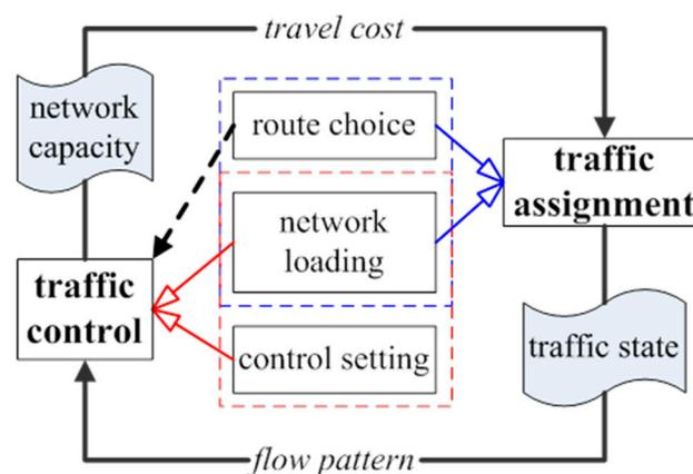
Figure 1. Interaction between traffic assignment and traffic control.
