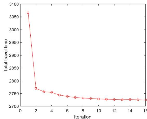
Figure 4. The convergence of the enhanced anticipatory traffic control algorithm.
