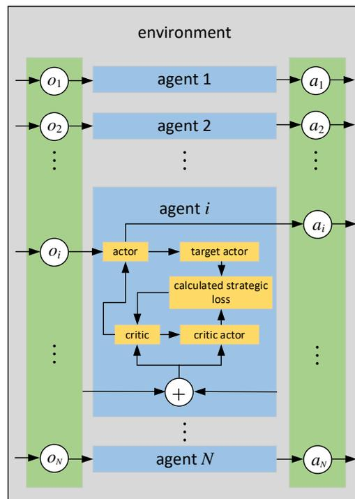
Figure 2. MADDPG algorithm training framework diagram.
