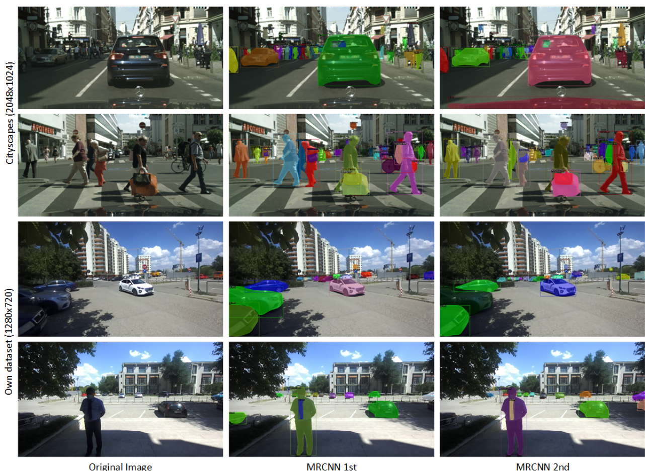
Figure 5. Mask RCNN output prediction examples on Cityscapes and our own images, MRCNN 1st —mask_rcnn_X_101_32x8d_FPN_3x, MRCNN 2nd —mask_rcnn_R_50_FPN_3x [42].
