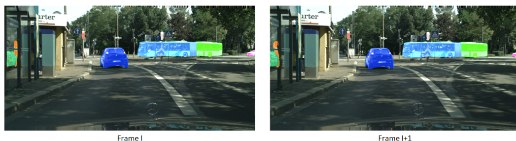
Figure 15. Wrong predictions propagation on the next frame: Mask RCNN prediction for Frame I , label and mask propagation using DIS for Frame I+1 .
