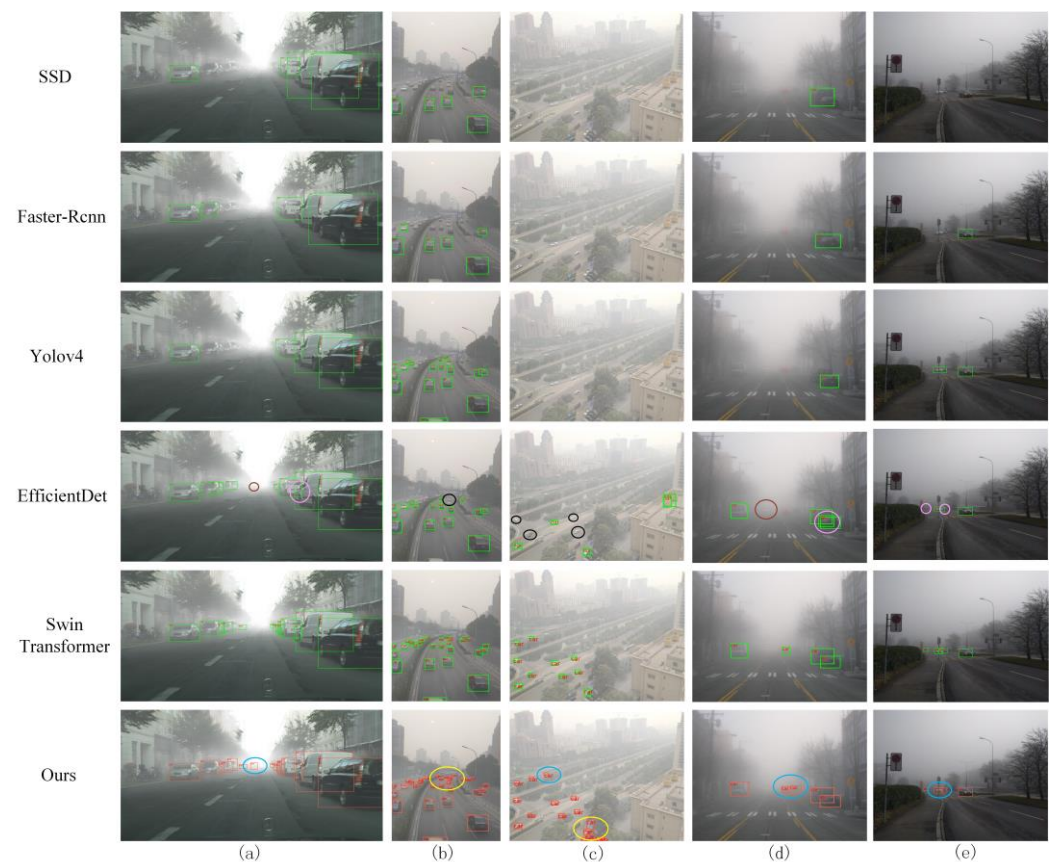
Figure 7. Qualitative comparison of detection results of our method and different algorithm models on the synthetic haze image Haze-Car (a–c) and the natural haze image Real Haze-100 (d,e).
