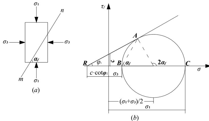
Figure 6. Mohr's circle when any point of the material reaches equilibrium state (a) microelement, (b) Mohr's circle.
