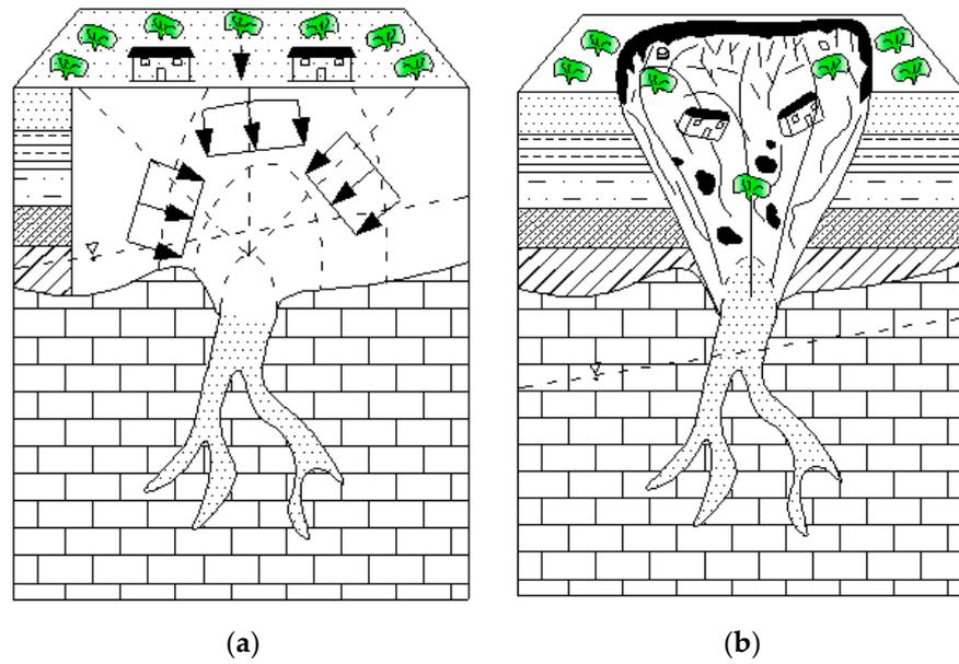
Figure 1. Limestone strata containing shallowly buried Karst caves. (a). Before collapse; (b). After collapse.
