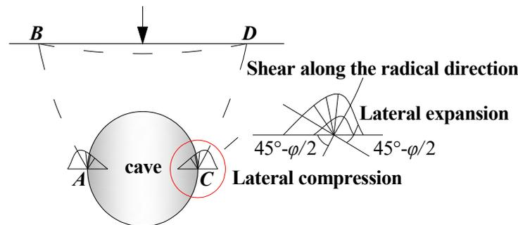
**Figure 4.** Vertical cross-section of limestone strata containing the spherical Karst cave, which was affected by the vertical load.
