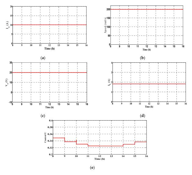
**Figure 6.** System dynamics using I/O linearization controller for: (**a**) Motor pump current, (**b**) motor pump angular speed, (**c**) motor pump voltage, (**d**) DC converter inductance current, and (**e**) control input stabilization.
