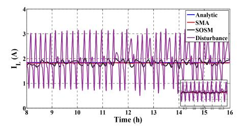
Figure 12. Inductance current of the DC converter under the indicated scheme.
