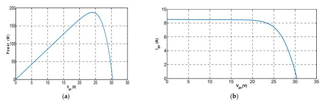
Figure 4. PV (a) and IV (b) characteristics of the PV module.
