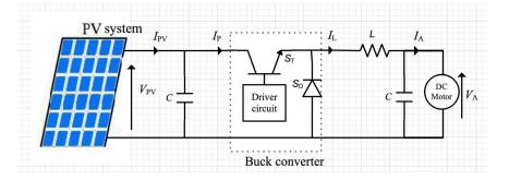
**Figure 3.** Electrical scheme of the studied system, where *C* is a capacitor, *L* is an inductor,  $I_L$  is the inductor current, and  $S_T$ ,  $S_D$  are a transistor and a diode of the step-down converter, respectively.
