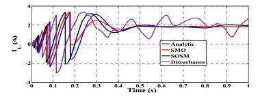
Figure 20. Inductance current of the DC converter for the indicated scheme.
