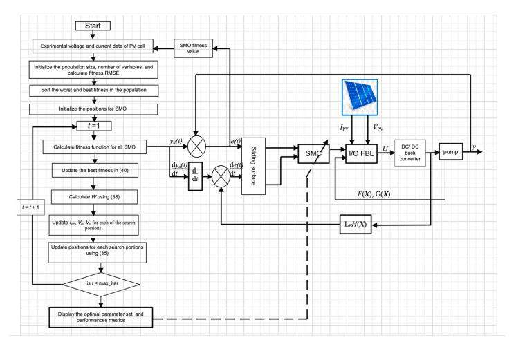
Figure 10. Block diagram of the SMO-SOSM-I/O FBL controller.
