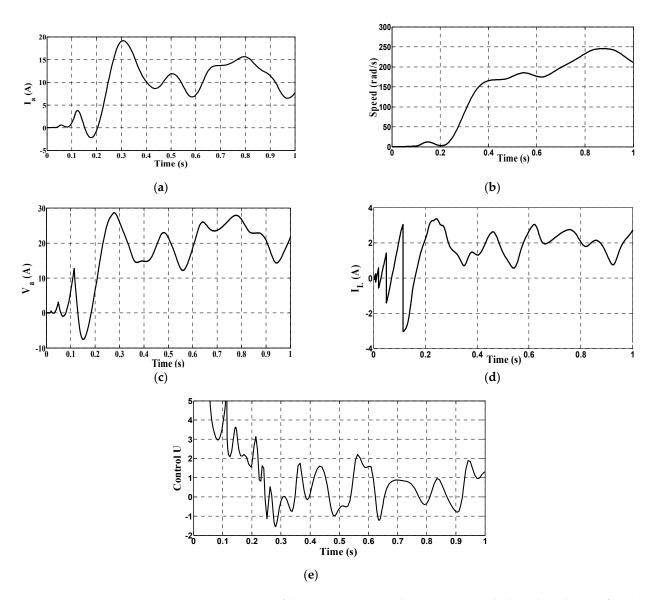
**Figure 18.** Dynamics of the motor pump with FBL control including disturbances for: (**a**) Motor pump current, (**b**) motor pump angular speed, (**c**) motor pump voltage, (**d**) DC converter inductance current. (**e**) control input stabilization.
