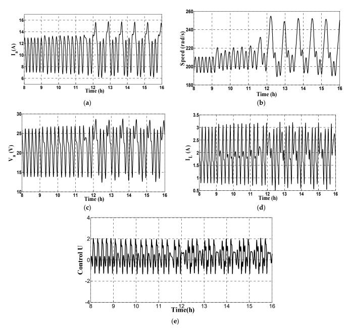
**Figure 7.** I/O control performance considering unmeasured random and matched disturbances for: (a) Motor pump current, (b) motor pump angular speed, (c) motor pump voltage, (d) DC converter inductance current, (e) control input stabilization.
