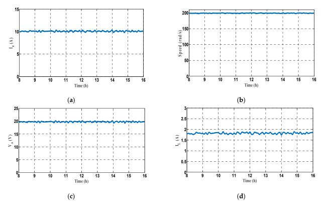
While the SOSM is applied to the approximation error, the PV system is controlled by the I/O linearization law described in (24). The consequential control performance is exhibited in Figure 8.
