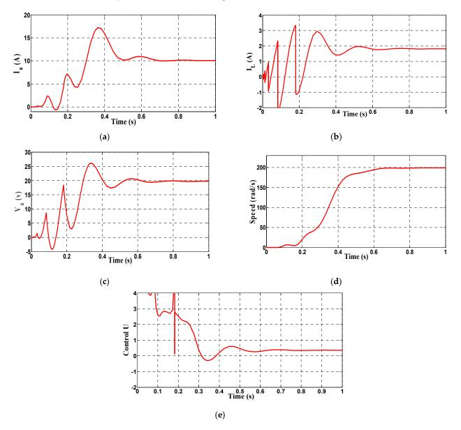
**Figure 17.** Dynamics of the motor pump with FBL control ignoring disturbances for: (**a**) Motor pump current, (**b**) motor pump angular speed. (**c**) motor pump voltage, (**d**) DC converter inductance current, (**e**) control input stabilization.
