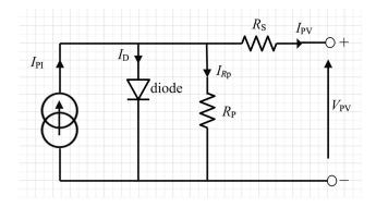
Figure 2. Electrical equivalent circuit of the PV cell.
