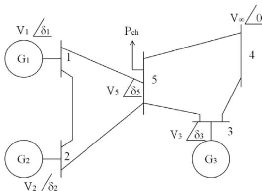
Figure 1. Three machine infinite buses.
