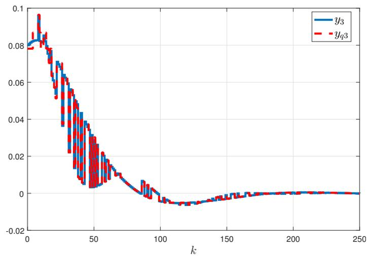
Figure 4. Actual output,  $y_3$ , and quantized output,  $y_{q3}$ .
