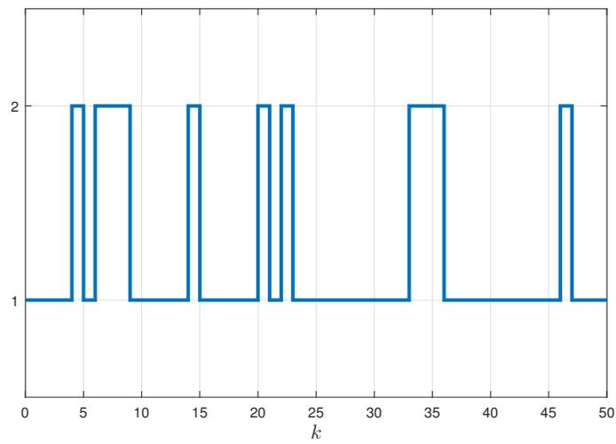
Figure 7. Mode values of Markov chains of an intermittent fault.
