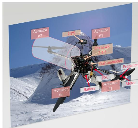
Figure 3. A real drone referenced in the paper.
