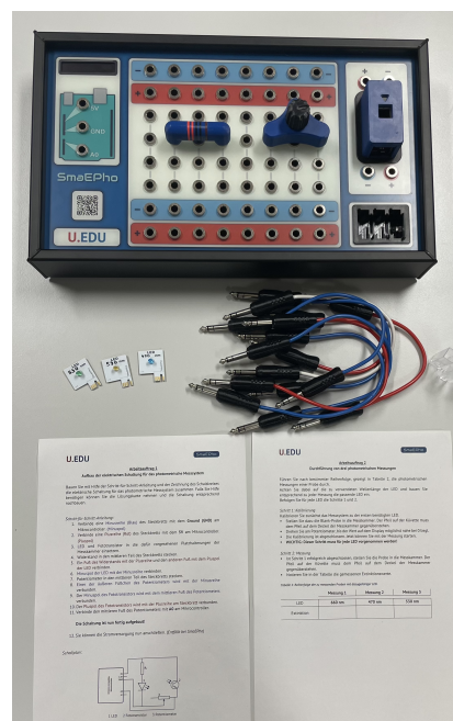
Figure 5. The system set-up for the usability evaluation of the SmaEPho including the SmaEPho, cables, LEDs, resistor, potentiometer, cuvettes, and the two worksheets with written instructions.
