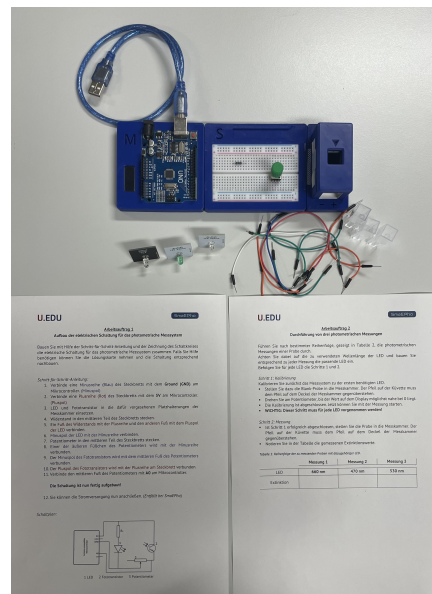
Figure 6. The system set-up for the usability evaluation of the desklab photometer including the desklab photometer, cables, LEDs, resistor, potentiometer, cuvettes, and the two worksheets with written instructions.
