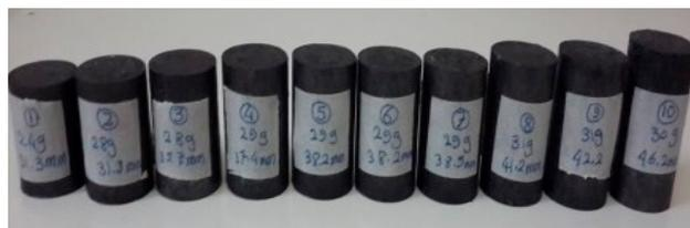
Figure 7. The produced samples using closed mold (D = 25, H = 50 mm).
