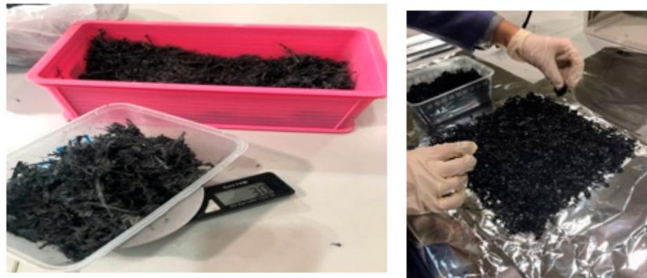
**Figure 1.** Shredded CFRP preparation for the autoclave process.
