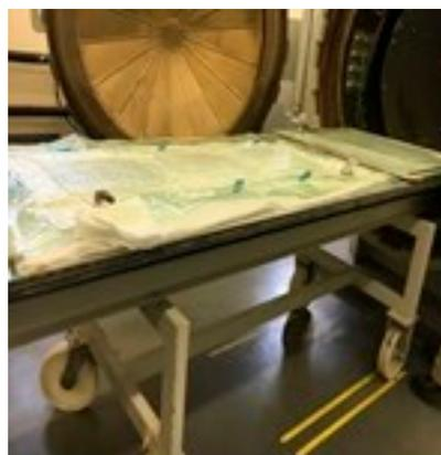
**Figure 2.** Autoclave to process the waste CFRP under the curing cycle.
