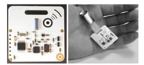
Figure 1. SocioPatterns sensor. Front aspect and scale.
