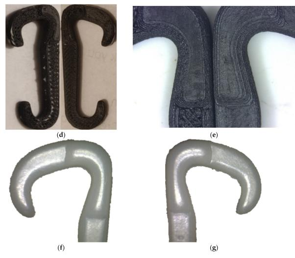
**Figure 1.** Surface finish of ring-spinning travelers; molded, chopped, fiber-reinforced G-77-C traveler (**a**), printed, plastic G-77-C travelers (**b**), printed, chopped, fiber-reinforced G-77-C traveler (**c**), printed, chopped, and continuous fiber-reinforced J-102-C traveler (**d**,**e**), and molded, chopped, fiber-reinforced J-102-C traveler (**f**,**g**).
