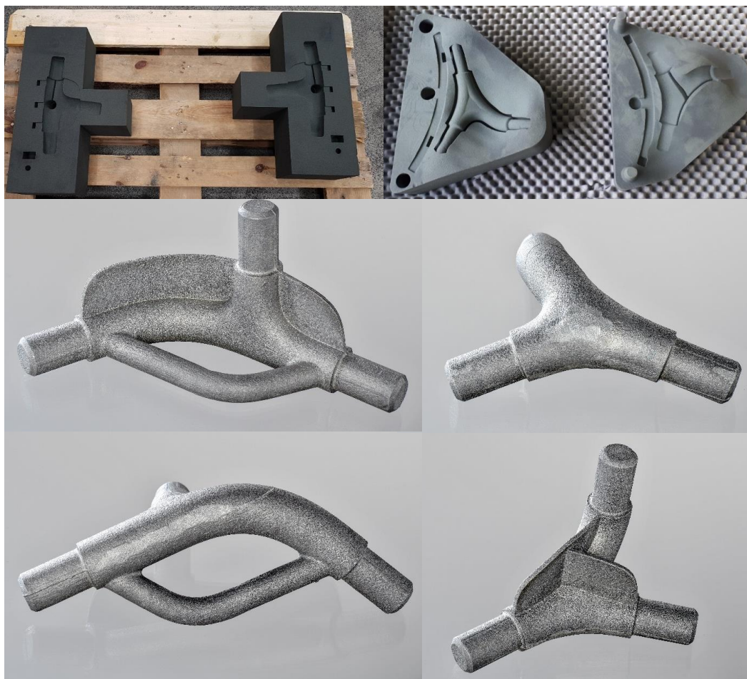
Figure 2. The upper row shows two printed mold parts for manufacturing the casting knots. The molds are mirrored to be used in the left and right side of the vehicle body structure. The lower rows present two sample functionally integrated casted knots for joining the tubes of the vehicle body. The passenger can use the additional strut (left knot) as a handle. The reinforcements of the left knot are the fixing points for the roof cladding and windscreen. The right knot joins the tubes at the car's entry.
