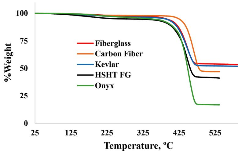
**Figure 2.** Thermo-gravimetric analysis (TGA) spectra of composite filaments.
