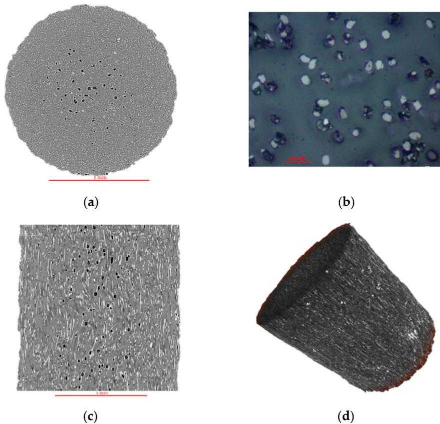
**Figure 3.** Different views of Onyx plastic filament: cross-sectional view from nano-CT scanning indicating fiber and void distribution (a), magnified (500×) microscopic view of the cross-section (b), longitudinal view from nano-CT scanning showing fiber orientation (c) and 3D view taken using nano-CT scanner (d).
