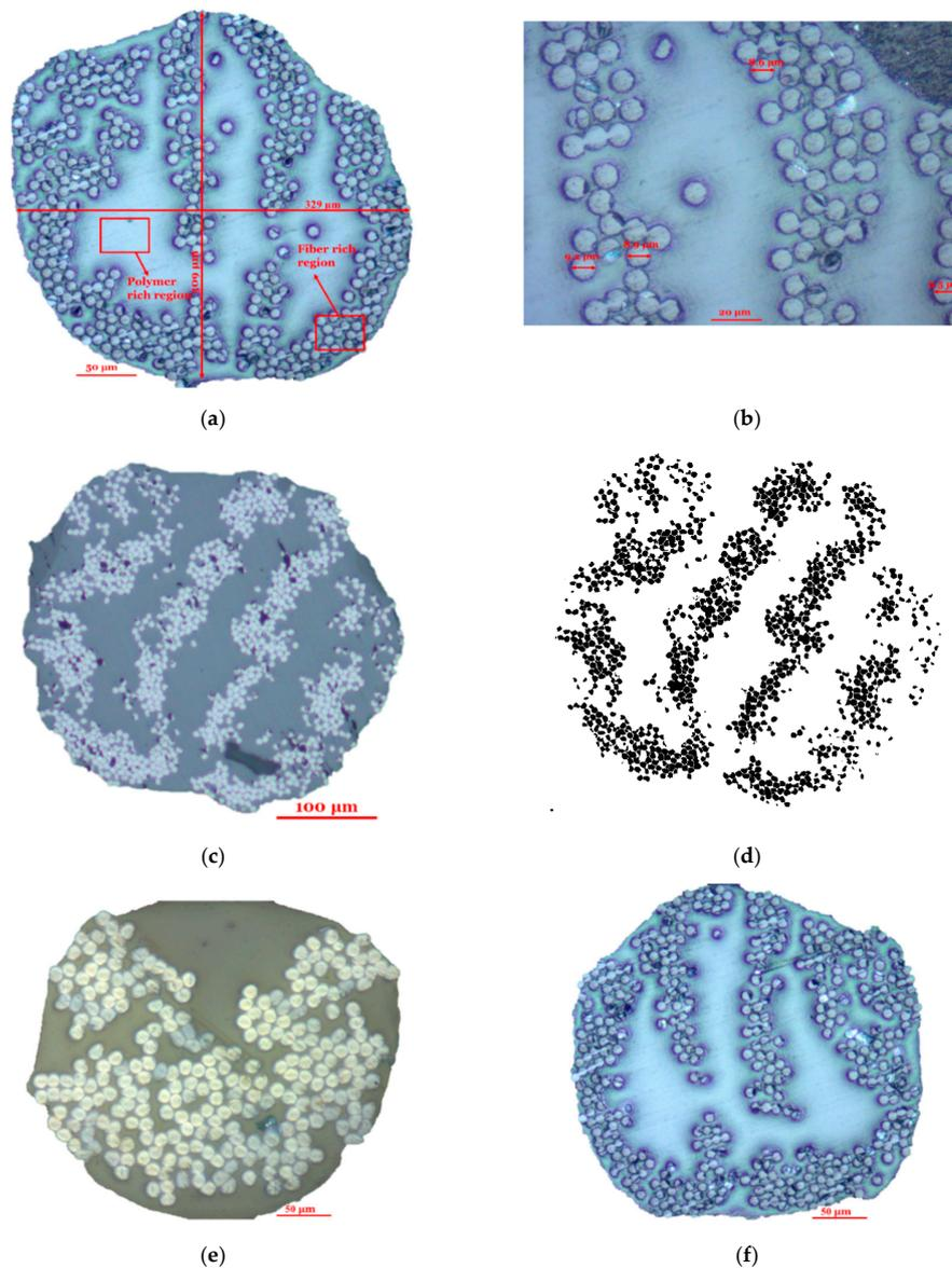
**Figure 4.** Cross-sectional views of fiber filaments (for fiber supply); fiberglass at 200× (a), fiberglass 500× (b), carbon fiber at 100× (c), carbon fiber filament tows shown as dots applying cell counting procedure using ImageJ (d), Kevlar at 200× (e) and high strength high temperature fiberglass (HSHT) FG at 200× (f).
