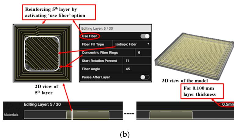
**Figure 5.** Interfaces of Eiger software for parameter setting and slicing: part view for parameter settings (a) and internal view for slicing as well as exploring different options for fiber-reinforcement (b).
