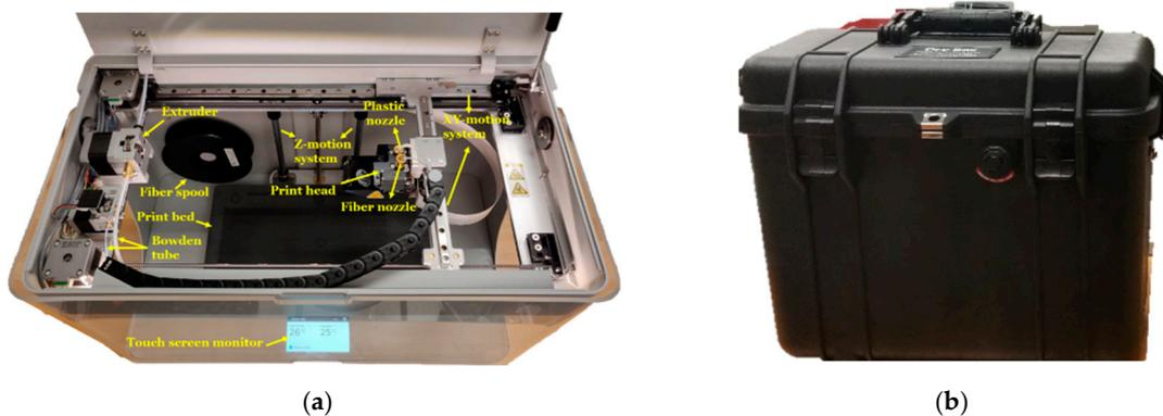
**Figure 1.** Mark Two 3D printer (desktop series) (a) and dry box to store and supply plastic filaments (b).
