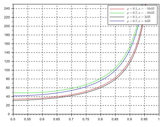
**Figure 9.** Average Delay (*D*) vs. transmission probability (*p*) using the second proposed backlog retransmission scheme for various values of correlation coefficient  $\rho$  and Rice factor ( $\kappa$ ).
