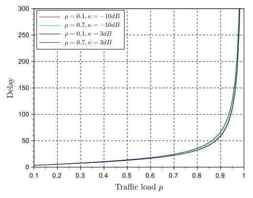
**Figure 8.** Average Delay (*D*) vs. transmission probability (*p*) using the first proposed backlog retransmission scheme for various values of correlation coefficient  $\rho$  and Rice factor ( $\kappa$ ).
