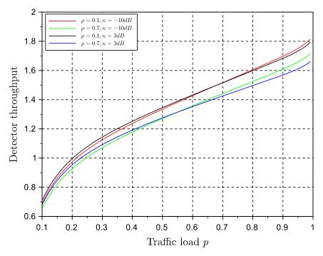
**Figure 7.** Stable throughput ( $T = \lambda J$ ) vs. transmission probability (p) using the second proposed backlog retransmission scheme for various values of correlation coefficient  $\rho$  and Rice factor ( $\kappa$ ).
