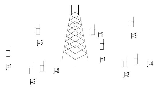
Figure 1. Random access wireless network scenario with MPR (M = 2).
