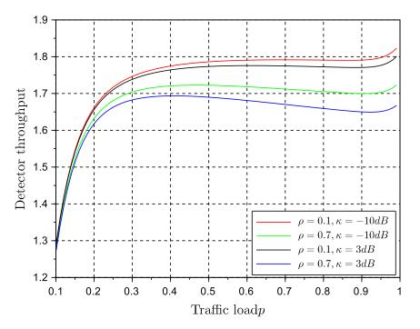
**Figure 6.** Stable throughput ( $T = \lambda J$ ) vs. transmission probability (p) using the first proposed backlog retransmission scheme (persistent) for various values of correlation coefficient  $\rho$  and Rice factor ( $\kappa$ ).
