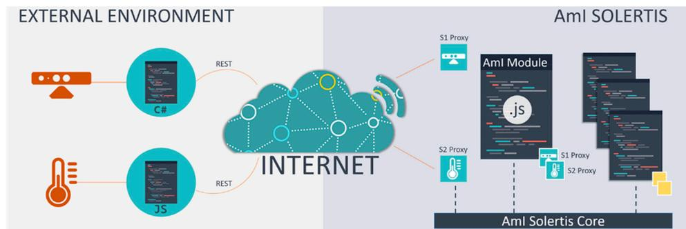
**Figure 1.** The AmI-Solertis Hybrid Communication Protocol.
