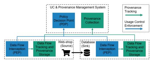
Figure 2. An exemplary data provenance and usage control architecture.
