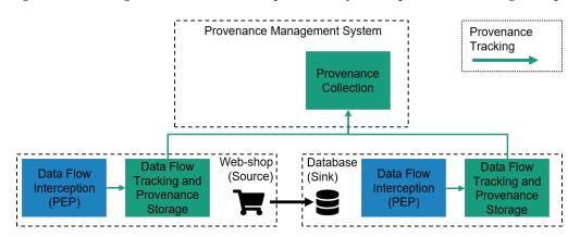
Figure 1. An exemplary data provenance tracking architecture.
