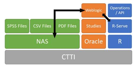
**Figure 4.** System structure for the current implementation of the proposal. The communication between the different subsystems is done mainly through the network attached storage (NAS), Weblogic and R-Serve packages that primarily serve as matrix, questions and operations managers.
