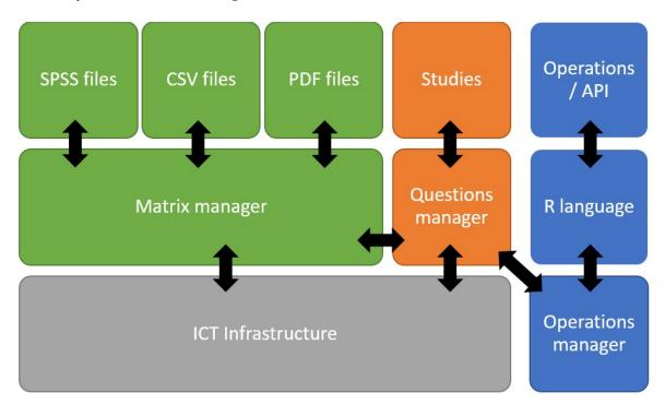
**Figure 3.** Proposed architecture for the management of statistical information. The Information and communications technology (ICT) infrastructure support the management of the information, while the operations manager supports providing calculus and the API to this information. This subsystem can be over the ICT infrastructure or be considered as a separate piece that uses an independent infrastructure.
