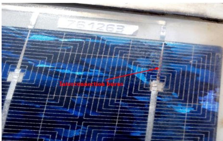
**Figure 6.** Module 10, indicating interconnection burns.
