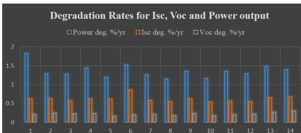
**Figure 10.** Degradation rates of 14 PV modules.
