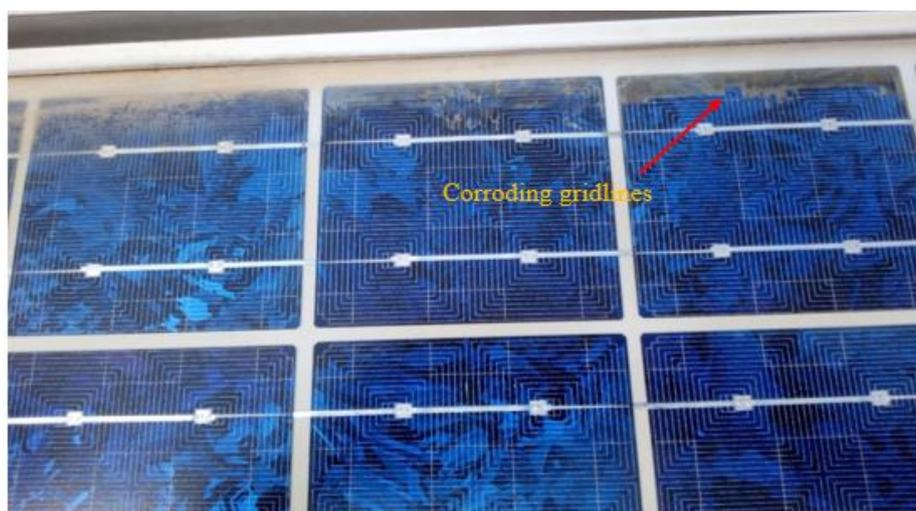
**Figure 5.** Module 12, indicating corroding gridlines.
