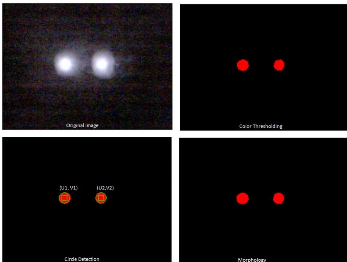
Figure 2. Blob detection and tracking algorithm outputs.
