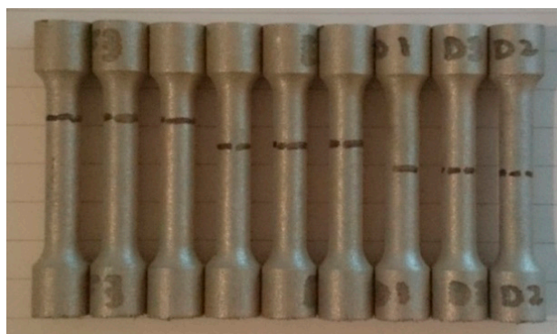
Figure 10. Customised specimen set failure points.
