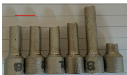
Figure 6. Set B (175 W) specimen fracture locations.
