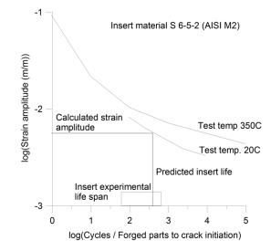
Figure 5. Illustration of the outcome of a local strain approach for damage analysis ref. [2].
