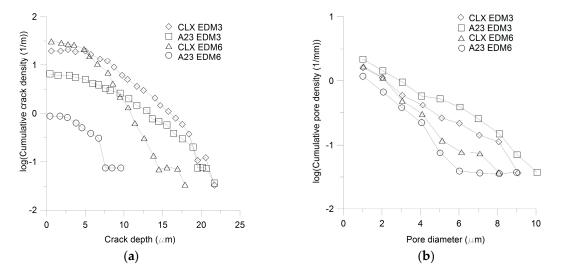
**Figure 13.** Defect distribution under different conditions for CALMAX(CLX) and ASP2023(A23), (a) cracks, after ref. [25] (b) pores after ref. [25].
