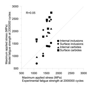
Figure 10. Failure reasons at various experimental strengths after ref. [23].
