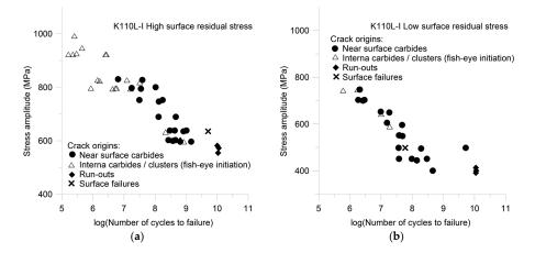
**Figure 8.** (a) Fatigue data of ultrasonic high cycle fatigue tests for AISI D2 steel K110L-I with high surface residual stress after ref. [20]; (b) Fatigue data of ultrasonic high cycle fatigue tests for AISI D2 steel K110L-I with low surface residual stress after ref. [20].
