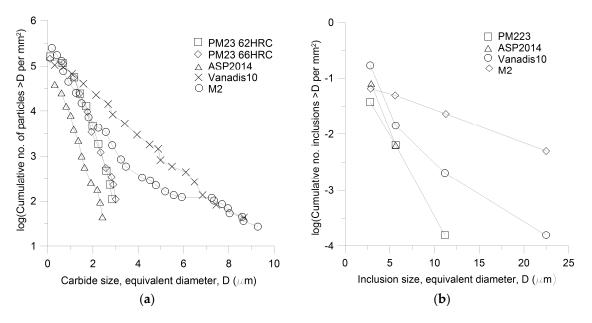
**Figure 11.** (a) Carbide size distribution for various tool steels [22]; (b) Inclusion size distribution for various tool steels [22].
