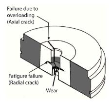
Figure 3. Typical locations of failures and their location in a die after ref. [3].
