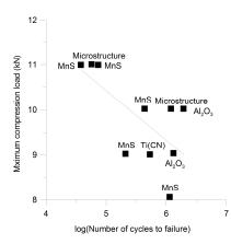
Figure 9. Reasons for fatigue failures in 100Cr6 high strength steel (martensitic bearing steel) after ref. [21].
