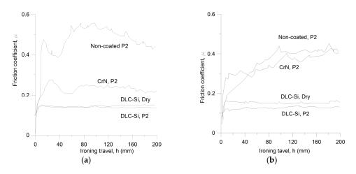
**Figure 15.** Variation of friction coefficient during ironing with a 20% reduction (**a**) SPFC590, after ref. [31]; (**b**) C2801-1/4H after ref. [31].
