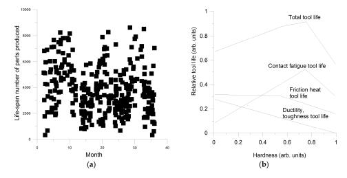
**Figure 1.** Tool life, (**a**) data of life spans of individual tool inserts over time illustrating the large variation observed under industrial practice conditions, after ref. [5]; (**b**) schematic relation between toll hardness and reasons for failure in tooling after ref. [6].
