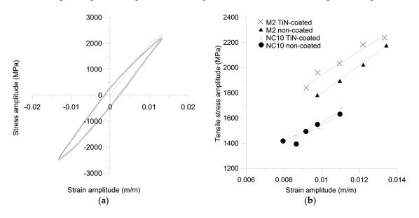
**Figure 20.** Material fatigue response (**a**) Hysteresis loop for non-coated M2 tool steel at a strain amplitude of 0.0135, after ref. [53]; (**b**) Material fatigue response, cyclic strain amplitude—strain curves after ref. [53].
