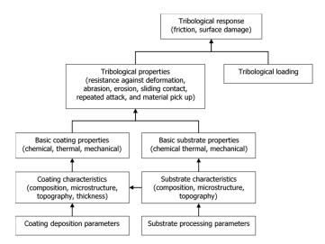
Figure 16. General relation between coating deposition and tribological response [36].
