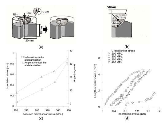
**Figure 17.** Illustration of layer adhesion testing, (**a**) Testing model; (**b**) stresses in the interface, after ref. [42] (**c**). Illustration of layer adhesion testing, Relation between initial delamination and assumed critical shear stress; (**d**) relation between length of delamination and indentation after ref. [42].
