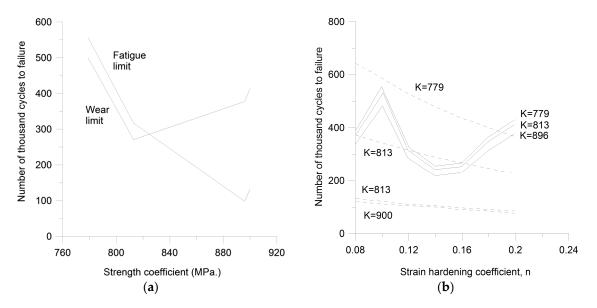
**Figure 6.** (a) Simulated fatigue and wear life versus strength coefficient after ref. [16]; (b) Simulated fatigue life for four different strengths coefficients versus the strain hardening coefficient after ref. [16]. Dashed line = fatigue limit, solid line = wear limit.
