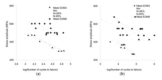
Figure 14. Fatigue life under different conditions (a) CALMAX(CLX) (b)ASP2023(A23) [25].
