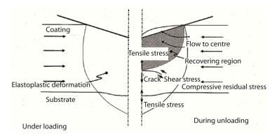
Figure 19. Model for coating fracture mechanism during indentation [44].
