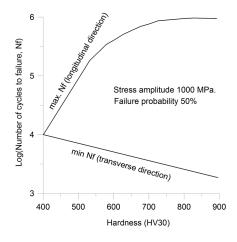
Figure 2. Material anisotropy effects in fatigue-life for tool steels after ref. [7].
