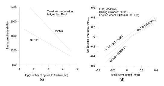
**Figure 7.** (a) Stress strain curves for M2 and D2 tool steels after ref. [2]; (b) Relation between hardness and tensile strength for SKD11 (D2-type) and QCM8 (low Cr version of SKD11) after ref. [18]; (c) Relation between stress amplitude and fatigue life for tension-compression fatigue for SKD11 (D2-type) and QCM8 (low Cr version of SKD11) after ref. [18]; (d) Relation between sliding speed and wear rate for SKD11 (D2-type) and QCM8 (low Cr version of SKD11) after ref. [18].
