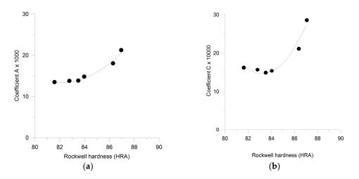
**Figure 18.** (a) Relationships between the hardness and the evaluated coefficient A and Rockwell hardness, after ref. [43]; (b) Relationships between the hardness and the evaluated coefficient C and Rockwell hardness after ref. [43].
