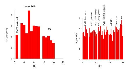
**Figure 12.** Stress intensity factors (**a**) found in three types of tool steels based on carbides after ref. [22]; (**b**) found in four different tool steels at different conditions, based on inclusions after ref. [22].
