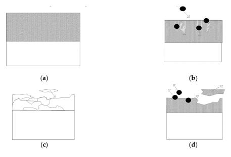
**Figure 21.** The four basic categories of tribological surface modification: (**a**) modification without any material transfer; (**b**) modification involving material transfer; (**c**) formation of tribofilm or coating; and (**d**) wear (loss of particles or atoms from the surface) [58].
