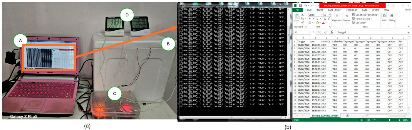
Figure 3. (a) Testing Setup; (b) Display and Data Logger of the Low-Cost Tropical Chamber.
