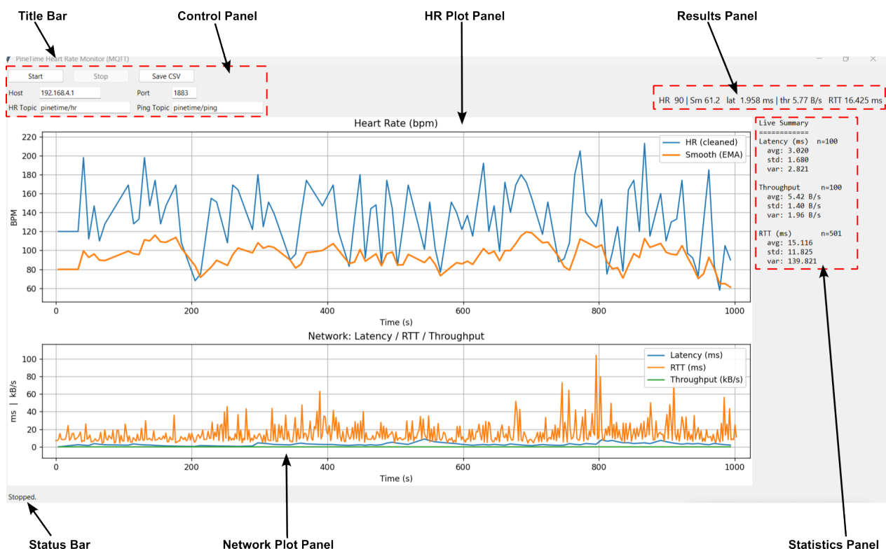
Figure 8. Application user interface with cleaned and smoothed graph of HR data.
