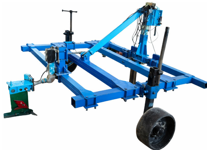
Figure 5. Installation of the L-shaped strain-gauge beam on the laboratory–field test facility for determining the draft resistance of the subsoiler.
