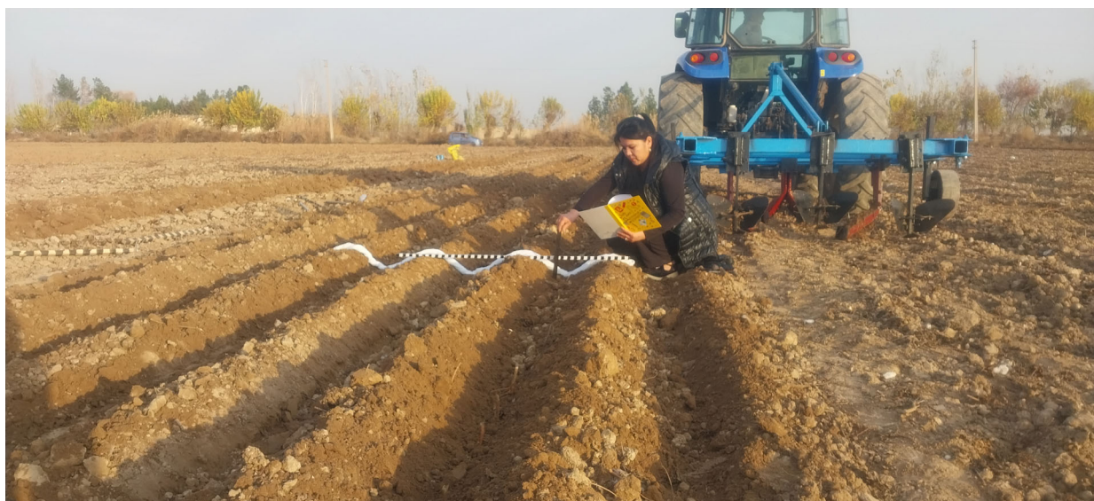
Figure 23. In situ procedure for verification of ridge geometry during the field validation trials: recording of the transverse ridge profile using a flexible profile gauge immediately after machine operation.
