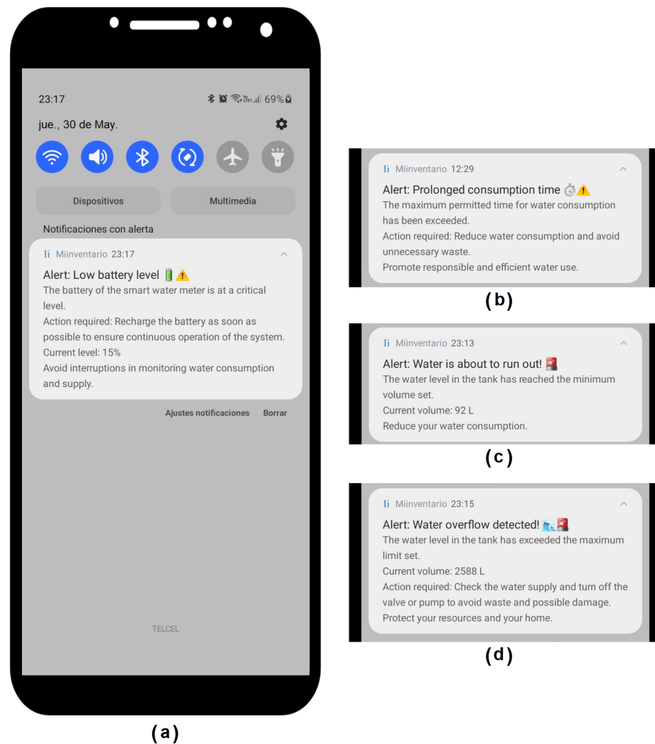
Figure 13. (a) Alert: Low battery level. (b) Alert: Prolonged consumption time. (c) Alert: Water is about to run out. (d) Alert: Water overflow detected.
