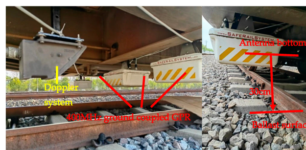
Figure 3. A subgrade condition inspection vehicle equipped with a three-channel GPR antenna array (reproduced from reference [14], licensed under CC BY 4.0).
