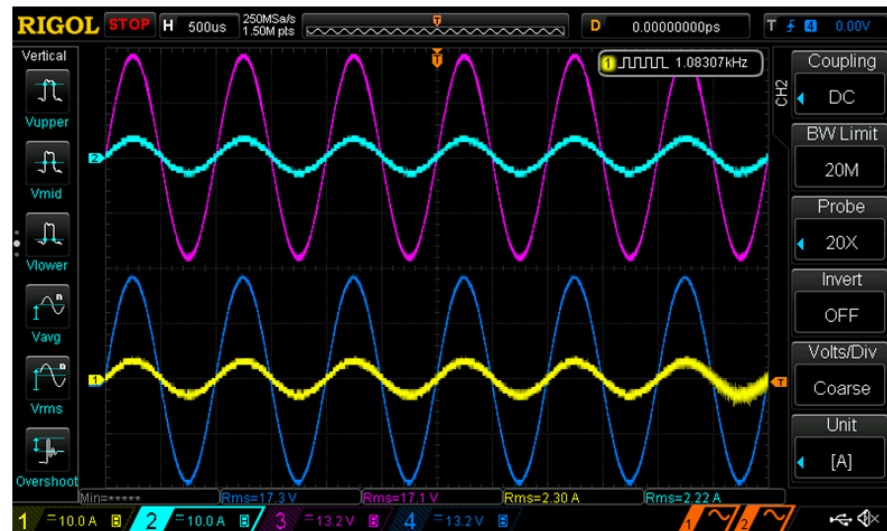
Figure 9. Oscilloscope capture for Output signals. (CH1—IOUT(L); CH2—IOUT(R); CH3—VOUT(R); CH4—VOUT(L)).
