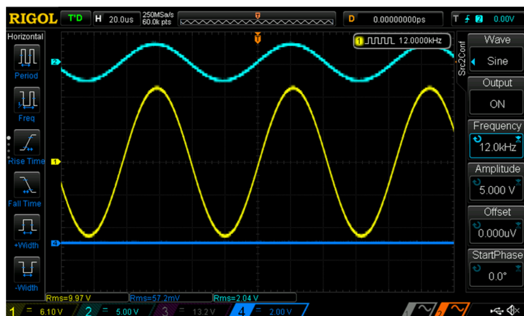
Figure 11. Oscilloscope capture for Frequency Response [ f = 12 kHz]. (CH1—Speaker output; CH2—Input signal; CH4—Subwoofer output).
