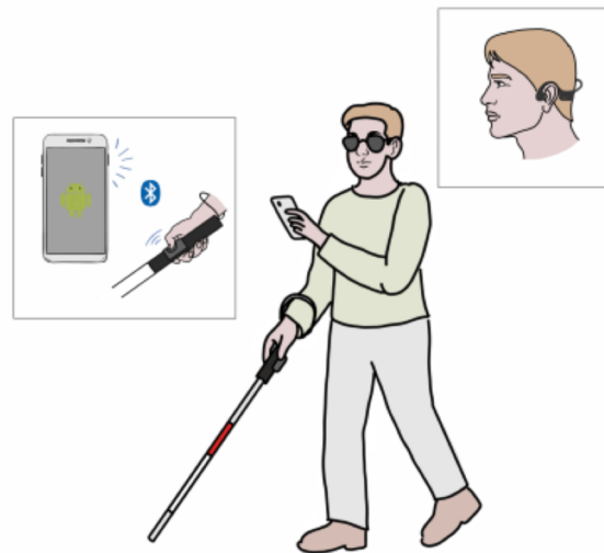
Figure 2. A sketch representation of the SnapStick system. The blind participant takes a picture with their smartphone by pressing the Bluetooth button attached to a commercial walking cane (see the left squared panel). The app elaborates the picture and provides an auditory description of it. The participant can safely listen to the description thanks to the bone-conducting headphones (see the right squared panel).
