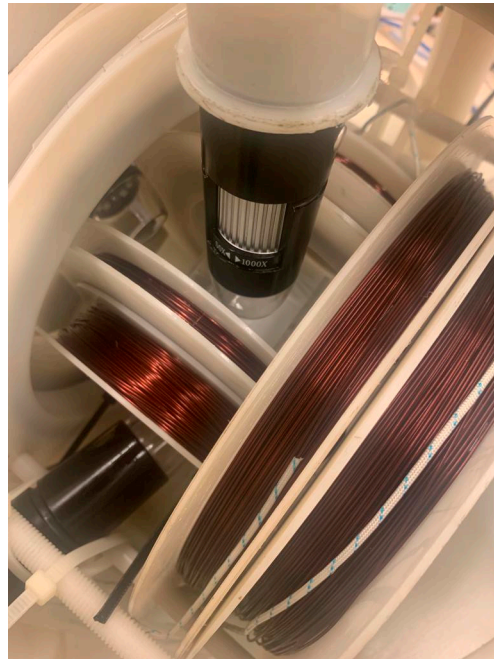
Figure 4. Microscope integrated with the EMA.
